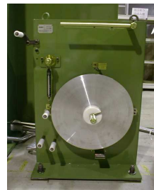
(Tape equipment) • Tape tension: Max.2kg • This tape is automatically controlled with hysteresis brake.
