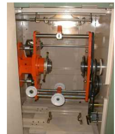
(J60H machine) • Lay length: 7.405~103.67mm • Tension equipment: hysteresis clutch
